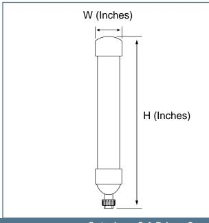
Truflo Calpro Series Calibration Columns have been Engineered to Measure the Flow Rates of Chemical Metering Pumps. The Calpro Series units provide an economical method for determining pump flow rate using standard graduations of milliliters | minute (ml/min) They offer accurate testing of metering pump flow rate by measuring the draw down rate on the suction side, while leaving the discharge undisturbed in its normal steady state operation condition.
